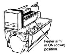
Depress water dispenser cradle for about two minutes to remove trapped air from water line and to fill water reservoir automatically. Ice cube mold automatically fills
